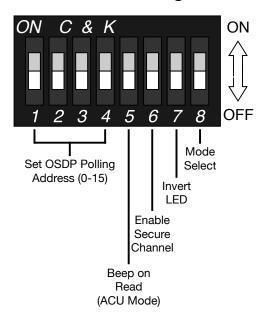
**DIP Switches 1-4:** Set the OSDP Polling Address in PD mode. Set the OSDP Address to be polled by the OSM unit in ACU mode. See the DIP Switch Address Table to the right.
